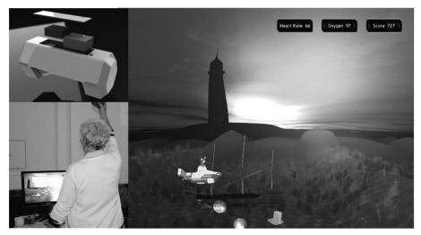
Fig. 3. Right: screenshot of the orange submarine game, top left: the dumbbell (exploded view, showing the accelerometer and pulseoximeter integrated), bottom left: person playing the game.
